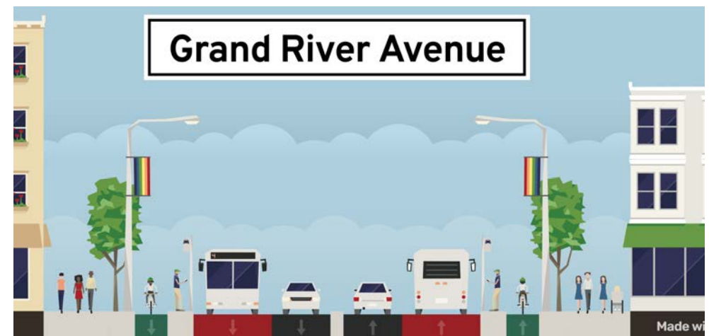
Figure 3-c: Mockup of potential street layout on Grand River Avenue, featuring protected bike lanes and a dedicated bus lane.
